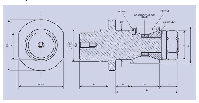
The clamping angles of mandrel and sleeve must be in permanent contact with each other for maximum efficiency.
